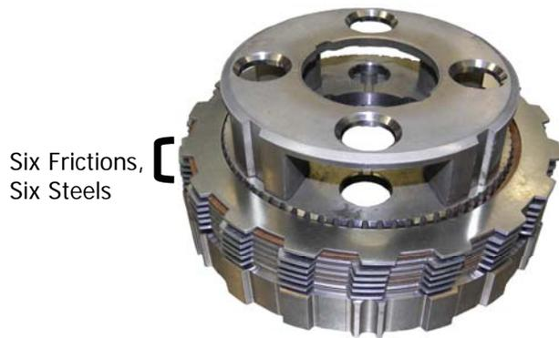
10. Install the clutch pack onto the planetary carrier. There are two stack ups from the factory; one with five clutches and one with six.
