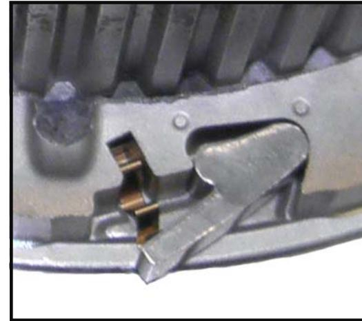
Load each pawl and spring like this. Put the spring side with three joints down (against the carrier).
