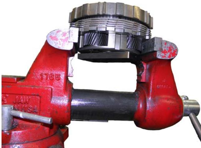
1. Install the drill jig into the planetary carrier from the front (diode) side of the carrier. Retain the jig in the carrier by placing the staking plate (plate pictured at left) on the bottom of the carrier and bolting the two together with the 3 1/2" long, 1/2"-13 bolt. Don't tighten the bolt at this point.
