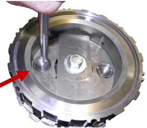
17. Loosen the clamping plate assembly and rotate it so as to support and expose the other two pins. Repeat steps 14, 15, & 16 for these pins.
