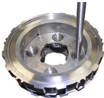
Check for movement in both directions, if pins aren't tight yet, if loose tap the pins forward before re-staking (drive as shown in picture at right).
