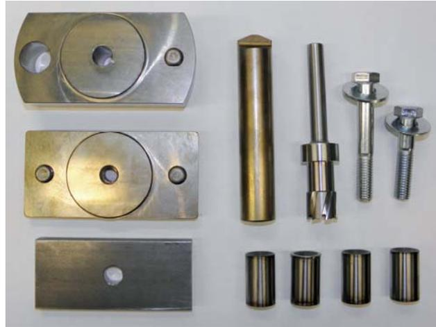
This tool is for use on **Ford Torqshift (5R110W)** transmissions.
