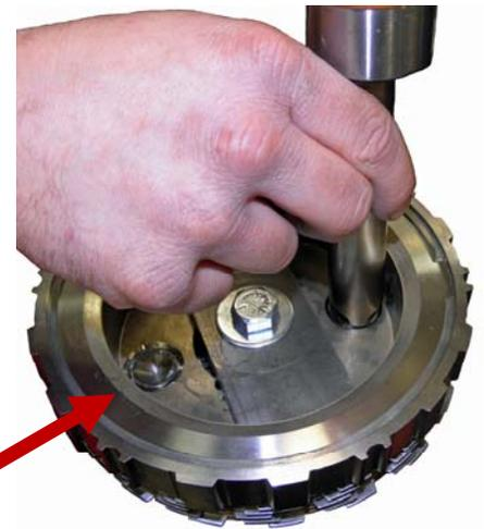
15. Take a drift punch (preferably 3/8" or slightly larger) and peen the head where you just swedged it. Care must be taken on this step not to excessively peen, as it is possible to crack the head of the pins.
