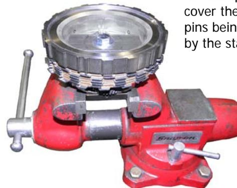
The two plates need to be at right angles to each other, otherwise the clamping plate will cover the heads of the pins being supported by the staking plate.
