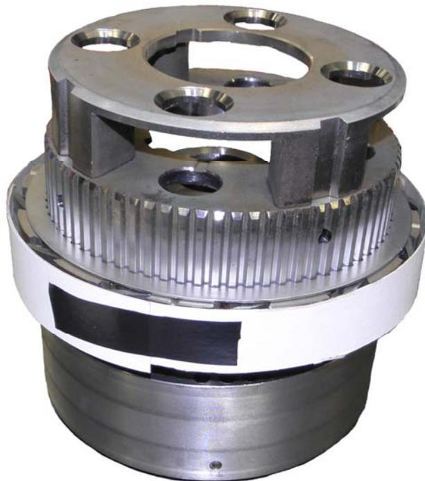
Left- Wrapped and supported carrier. Notice the thrust washer
