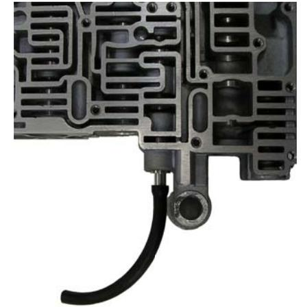
Sometimes the new throttle valve can be a little sticky. When you run into this, first check the valve for burrs, then stroke it in the bore to free. Vacuum line works great.
