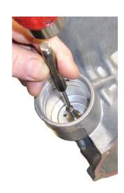
8. Insert the provided sizing pin into the bore, chamfer first. It may be necessary to start the pin in the bushing with a rubber mallet. Once the pin is inside the bushing, use a punch to drive the pin all the way through the bushing. The included sizing pin is larger than the factory servo pin, so repeat until the factory servo pin moves freely through the bushing.
